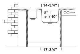
**Installer Notes:** Ukinox always recommends that you give the sink to the granite fabricator. If you are going to use a cutting board, provide that to the fabricator as well. Please note that we do include a template with each sink, but there can always be a slight variation. In addition, many of our templates are perforated so you can tear off the perforation for cutting board applications.
